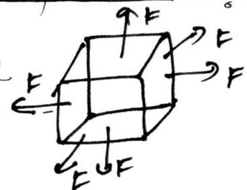
$$\boxed{\text{Bulk modulus } (K) = \frac{\text{normal stress}}{\text{volume strain}} = -\frac{F/A}{\Delta V/V} = -\frac{FV}{AV} = -\frac{PV}{V}}$$
