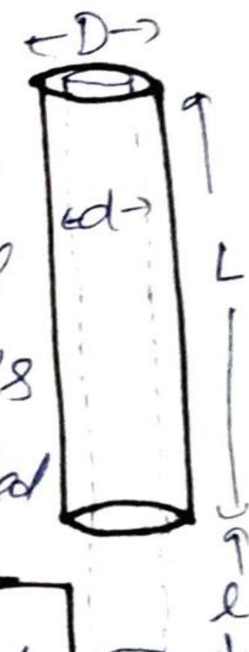
$$\sigma = \frac{\text{Lateral strain}}{\text{Longitudinal strain}} = -\frac{d/D}{\ell/L} = -\frac{Ld}{D\ell}$$
