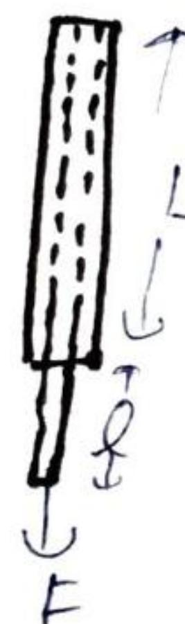
Young's modulus for a material is the force required to increase unit length of wire of unit area of cross-section by unity.
